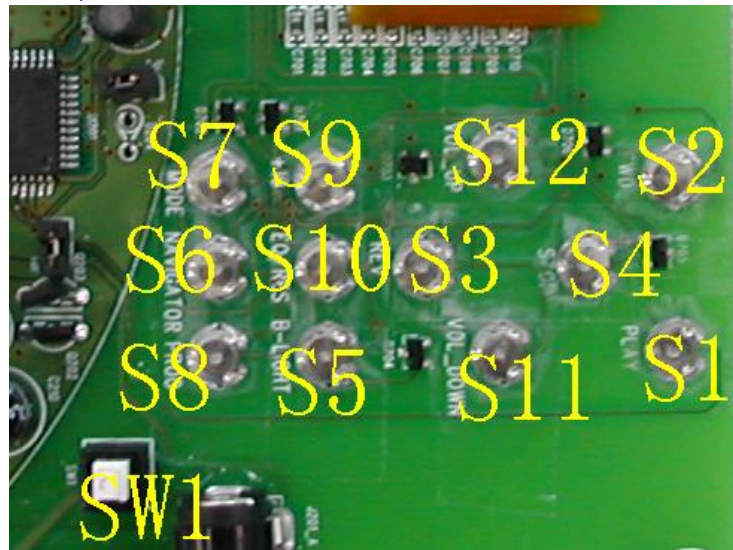
Figure 1-6. Detail View of the Button and Switch Matrix, from the Processor Board
